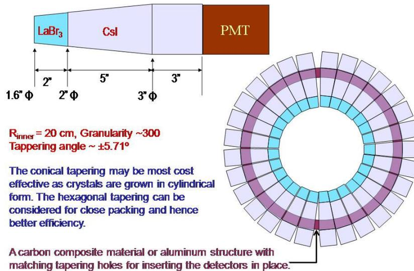
Tapering can be extended to the full length of the detector as shown below. There are various possibilities to choose depending on the availability of detectors and the cost involved. Some of the possible options are mentioned below.
