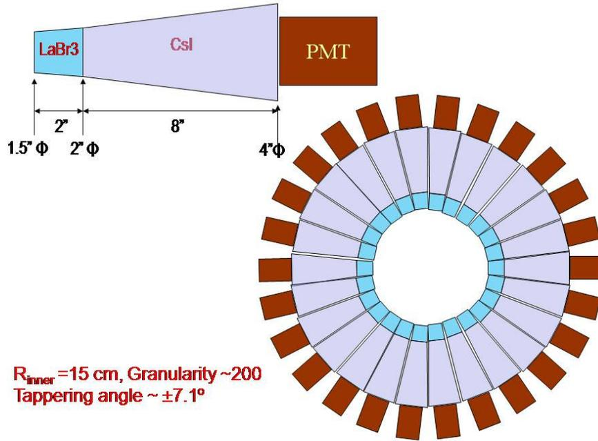
Higher inner radii is preferable and suppose we do not go for larger LaBr3 then one optimum option is the following geometry where 2" diameter LaBr3 is not tapered.
