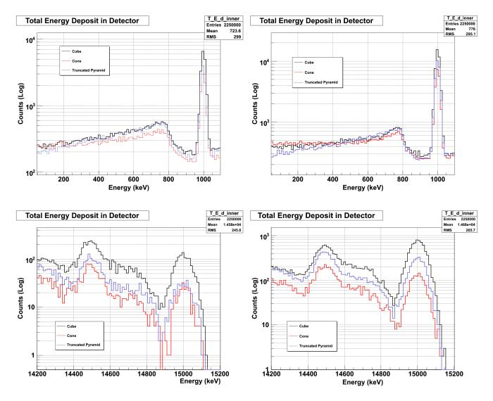
For the higher energy gammas (in our case 15MeV), we see that the cone produces good resolution in comparison to the other geometries, but a poor count rate. This is due to the very small face that was
