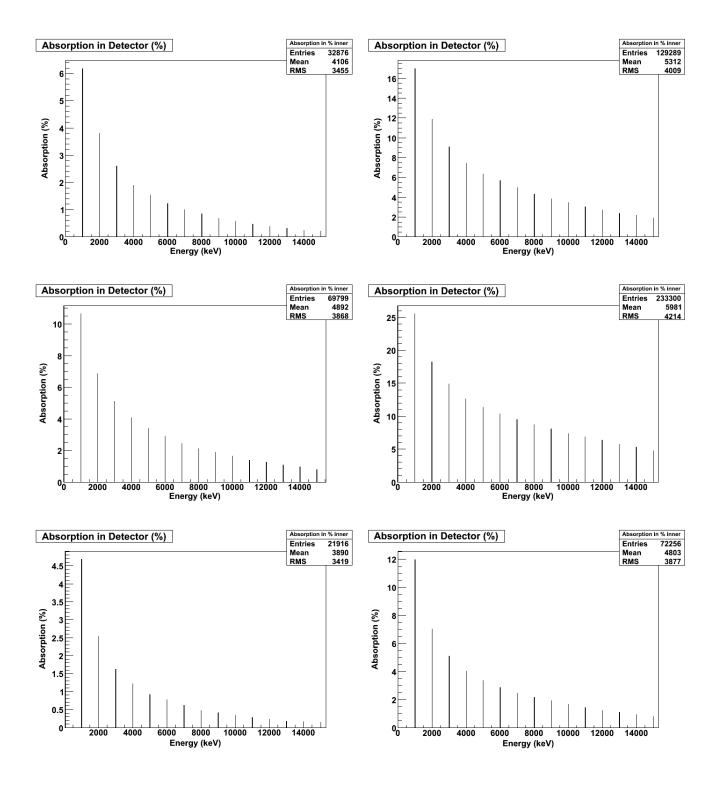
The graphs are laid out so that the first column are the smaller 1"x1"x4" measurements and the second column are 2"x2"x4" measurements, both easy to distinguish due to the increase in absorption efficiencies that one would expect foran extended volume size. The first row are the trapezoid/truncated pyramidal absorption graphs, followed by the cubic graphs in the second row and the cone measurements in the bottom row.
