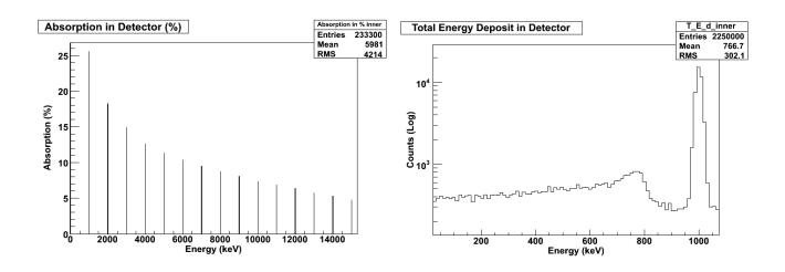
As one can see, the absorption is much higher than the previous simulation using this geometry. We now see a peak of  $\sim$ 25% at 1 MeV where a quarter of all gammas incident upon the crystal at this energy are absorbed. At 15 MeV, we see  $\sim$ 6-7% absorption, which again, is a vast improvement from the previous measurements. The spectrum is better too. The escape peak is more well defined instead of looking like "bump", meaning better resolution.
