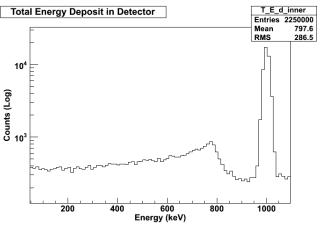
The top left graph is the Energy resolution of a 2"x2"x4" cube. The graph on the top right (above) is the energy resolution spectrum for a 1MeV gamma incident on a cone with inner diameter of 2". The last spectrum below (left) is a spectrum for the same incident energy but onto a truncated pyramid shape whose frustum measures 2"x2" in area. All the lengths of these solids were kept fixed at 4".
