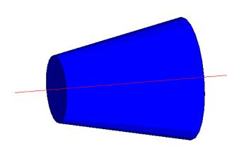
with the top cut offrevealing a frustum with a diameter of 2.54cm for the plane incident to the source. The bottom of the cone has a diameter of 4.62cm, which was calculated so that he projection of the beam followed the geometry of the cone, as was done previously with the other two designs. The length is 4" long to keep close to what was calculated with the trapezoid and cubic geometries.
