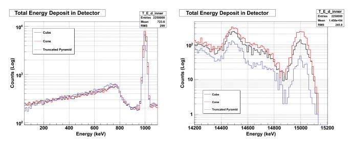
higher energies the trapezoidal shape is extremelypoor compared to the cone and cubic geometries.
