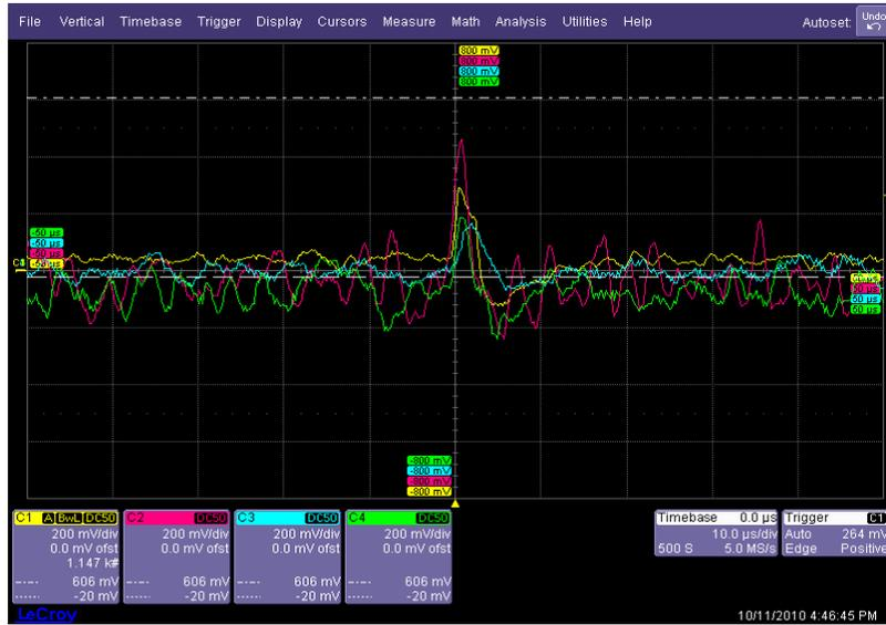
Figure 5.10: Gain-matching process, with radiation incident primarily on the second array/channel.
