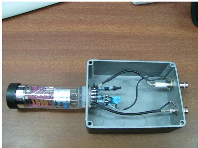
Figure 2.5: The constructed voltage divider
