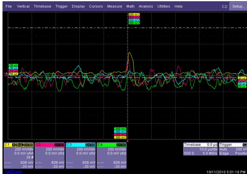
Figure 5.9: Gain-matching process, with radiation incident primarily on the first array/channel.
