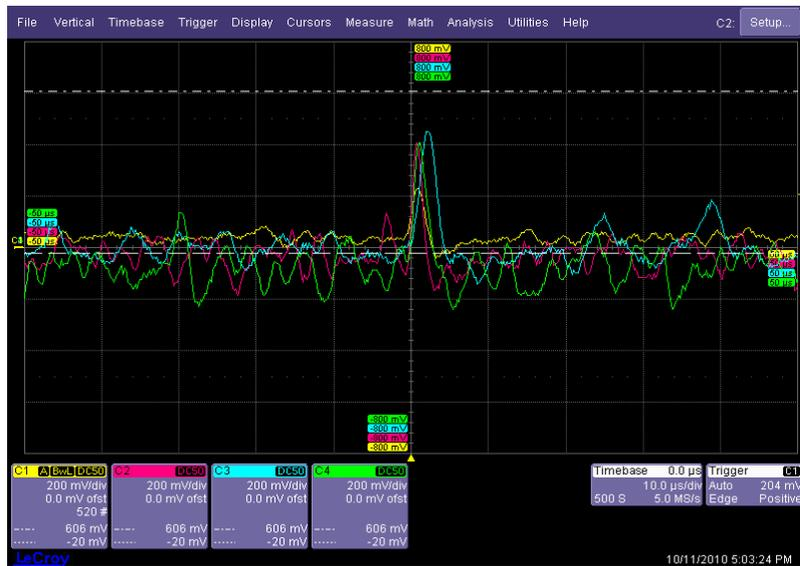
Figure 5.11: Gain-matching process, with radiation incident primarily on the third array/channel.
