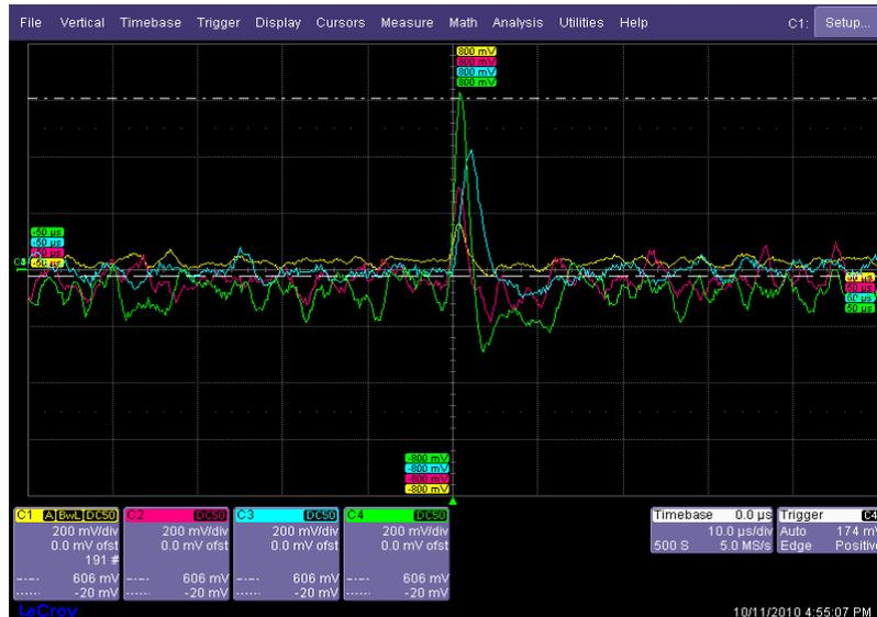
Figure 5.12: Gain-matching process, with radiation incident primarily on the fourth array/channel.
