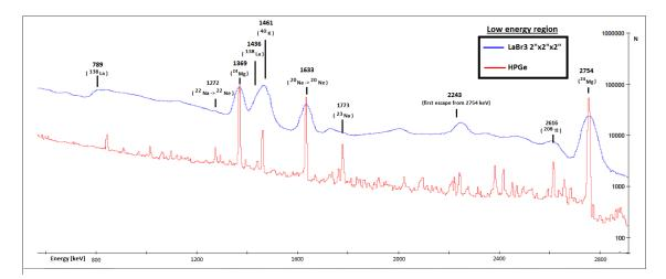
Fig. 2: Comparison of the spectra from cubic LaBr3 crystal (blue) and from the HPGe detector (red).
