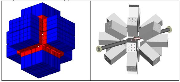
**Fig. 3**: Quasi-cubic (left) and quasi-spherical (right) PARIS geometry, made of 9-module clusters of phoswich (Labr3+CsI) detectors.
