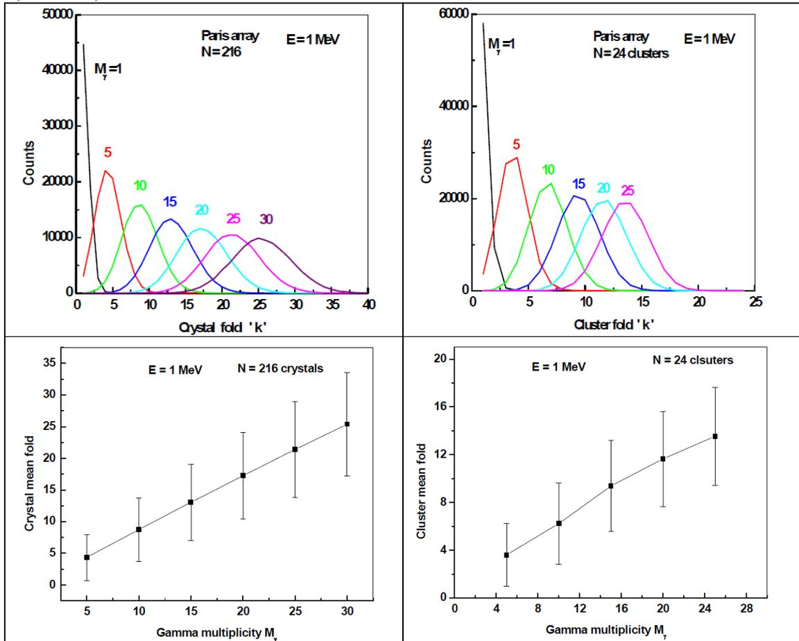
**Fig. 4:** Simulation of the multiplicity response of the quasi-cubic array (see Fig.3, left), consisting of 216 phoswich detectors arranged in 24 clusters of 9 crystals each.
