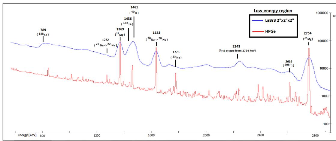
**Fig. 2:** Comparison of the spectra from cubic LaBr<sub>3</sub> crystal (blue) and from the HPGe detector (red).
