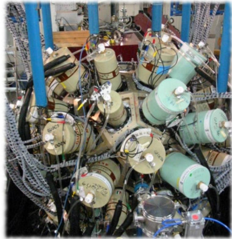
array of 43 Compton-suppressed HPGe detectors
